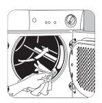
The filter in the inner door must be removed for cleaning.
